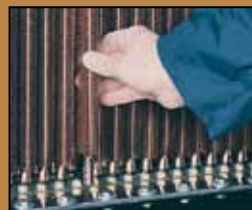
Tube is removed from header plate.
